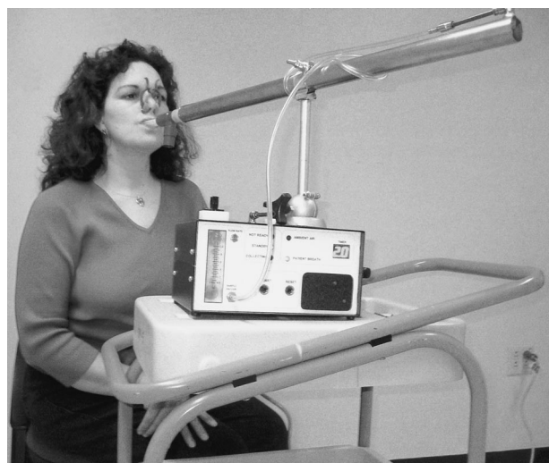
FIGURE 2. The breath collection apparatus is shown in use. The subject wears a nose clip and breathes quietly in and out through a disposable mouthpiece. The long tube is the breath reservoir, and the small tube affixed to its end is the sorbent trap, which captures the VOCs in the breath. The front panel of the breath collection apparatus shows the flowmeter on the left and a digital timer on the top right.
